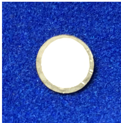
Figure 3.2: Thickness vibration mode disk-shaped BNBTM transducer; 8.4 mm diameter; 0.5 mm thickness
