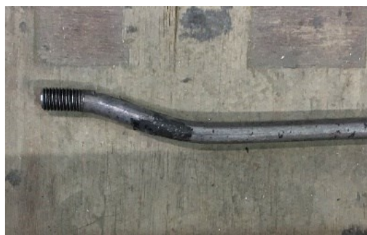
写真 2.4 4T16B120NN 芯材丸鋼の座屈
