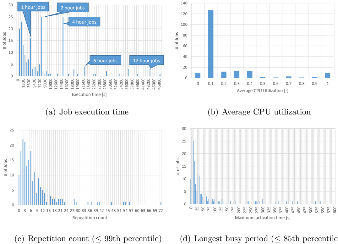
Figure 6.3: The primary statistics of interactive jobs collected on TSUBAME3.0. The sample size is 193 (jobs).
