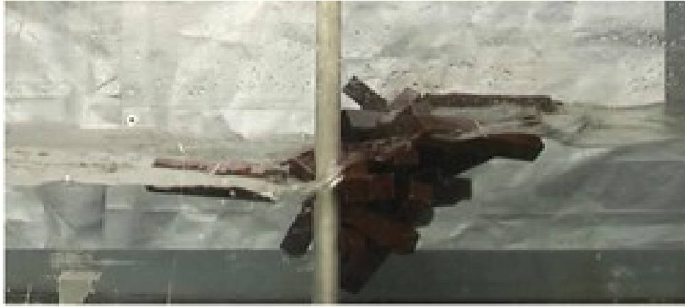
Figure 4.11: Experimental snapshot of the water surface and driftwood accumulation around poles at 14.8 s.
