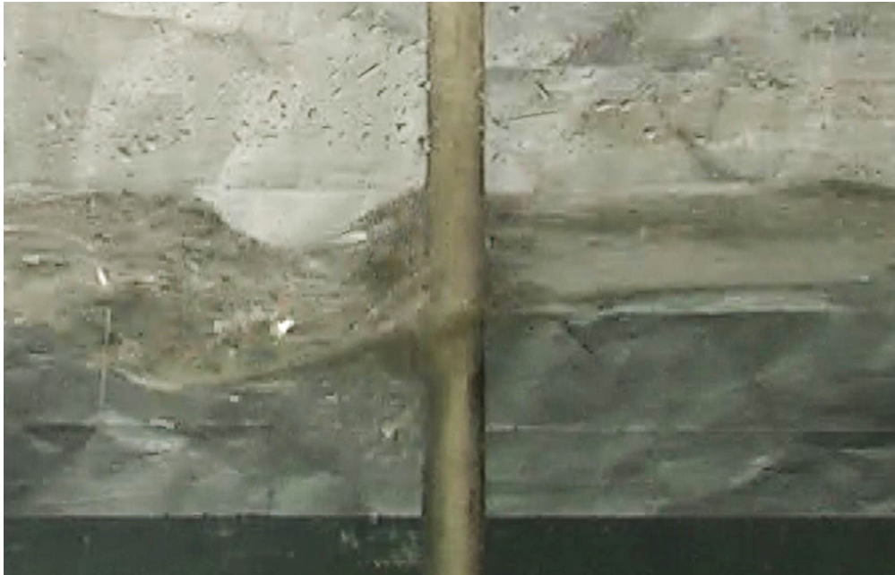
Figure 4.5: Water surface around poles of the experiment without driftwood at 19.5 s.
