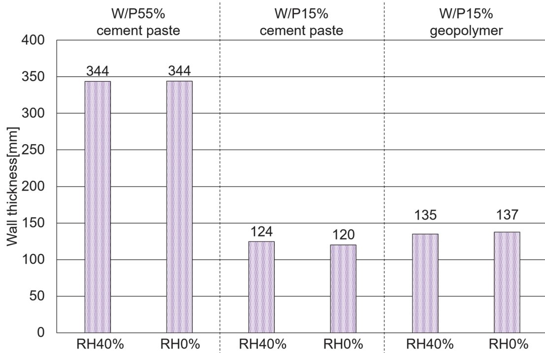
Figure 2-30 Calculated wall thickness of W/P55% cement paste specimen, W/P15% cement paste specimen and W/P15% geopolymer specimen at RH40% condition and at RH0% condition
