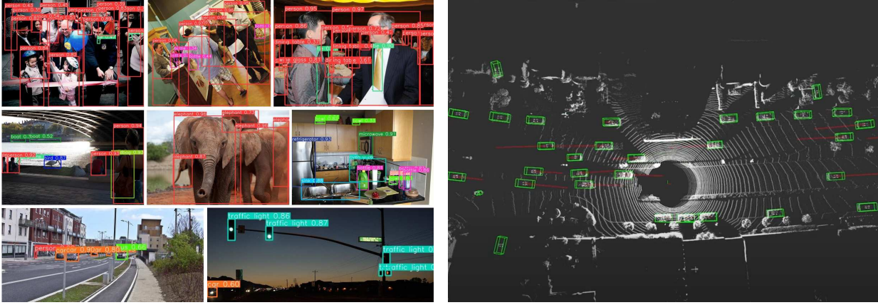
(a) Camera-based object detection with YOLOv10 (b) LiDAR-based object detection with CenterPoint
