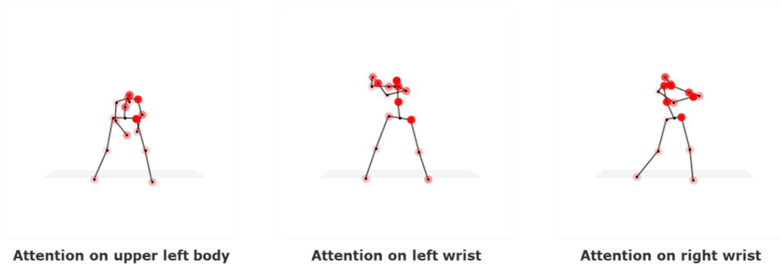
Figure 5.37: Visualization of body parts for revision suggestions. The attention-based network focuses on different body parts at three different phases (address, top, follow-through from left to right). The density and radius of red spheres show the intensity of the attention of the network.
