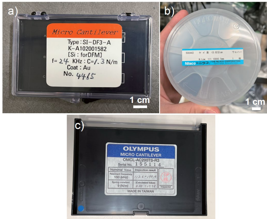
Figure 2.4 (a) Cantilevers (SI-DF3-A, Seiko Instruments Inc.), (b) Si wafer (SI-500443, Niraco Inc.), and (c) cantilevers (AC200TS, Olympus Inc.) used in the present study.
