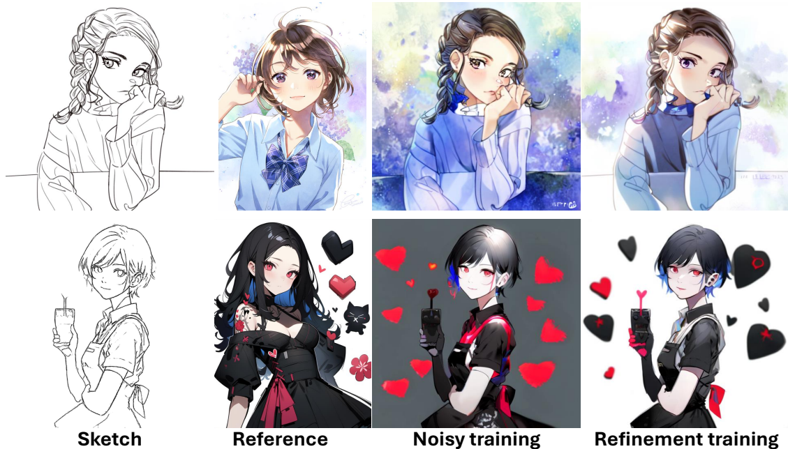
Figure 5.7: The color synthesized by the noisy-trained model is visually flat. Therefore, a refinement stage fine-tuning is adopted to fine-tune the transfer of color details.
