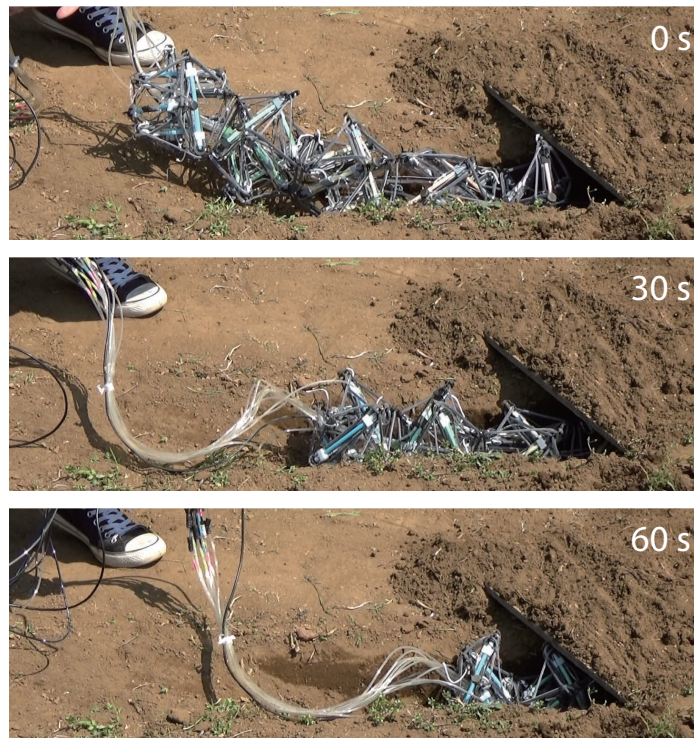
Fig. 4.7: Behavior of the tensegrity robot inducing propulsion from contact with a mud wall.
