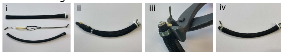
Fig. 5.9: Fabrication method of lossless stretchable McKibben muscle. (A) Fabrication method of inserted thread. (B) Fabrication method of rubber tube. (C) Fabrication method of sleeve. (D) Assembling of artificial muscle.
