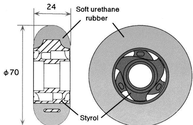
Fig. 18 Geometry of the wheel used for measurement
