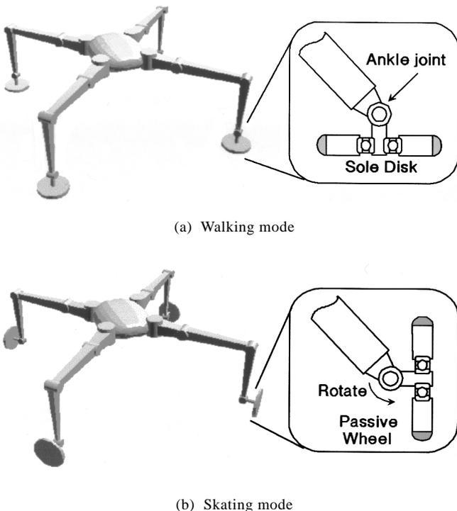
Fig. 2 Basic concept of Roller-Walker in two modes
