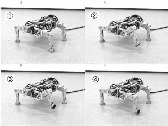
Fig. 14 Sequence of ankle turn over motion
