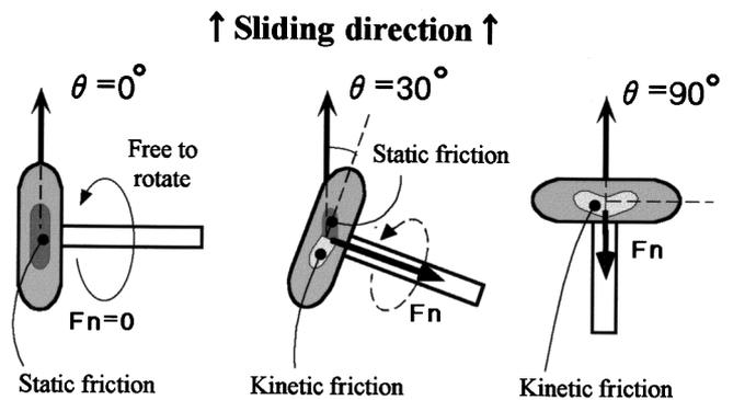
Fig. 21 Static/kinetic friction state at the contact point
