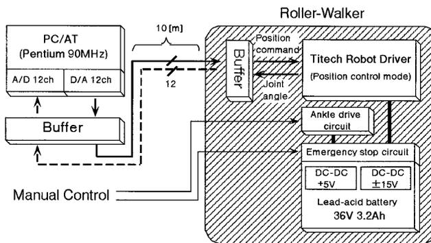
Fig. 12 Configuration of the control system
