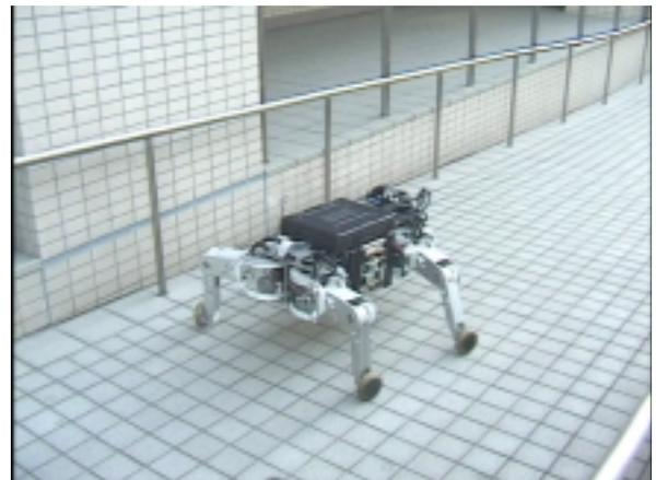
Fig.5 Slope climbing experiment
