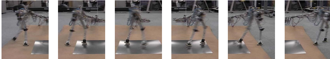
Fig. 6 Snapshots of a walking experiment over surfaces with different friction properties.
