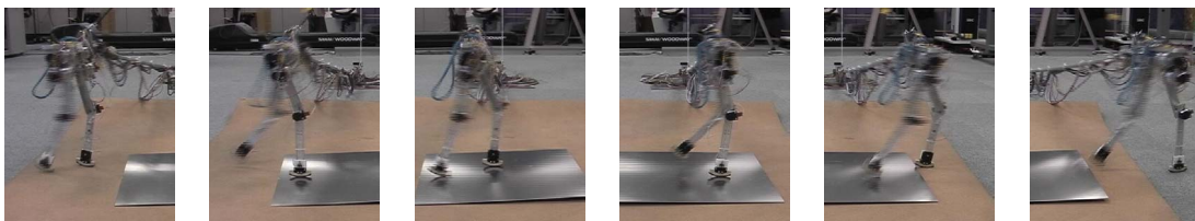
Fig. 7 Snapshots of a walking experiment over surfaces with different friction properties and a seesaw-like metal plate with a slight change in the slope.
