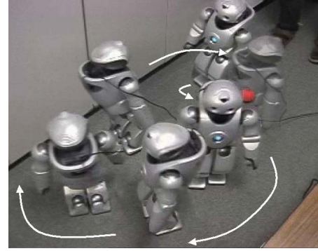
Fig. 15. Manueuvring experiment using combination of CPG and state-machine controller
