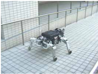
Fig. 6. Achievement of slope climbing propulsion ( \theta_0 = 0.4rad , \omega = 2.88rad/s , V = 0.32m/s )
