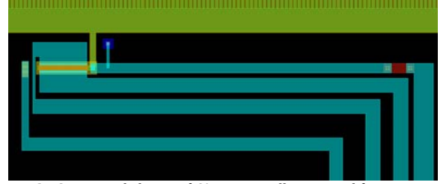
Fig. 3. One example layout of 60 automatically generated for a test chip experiment spanning 18 design variables.
