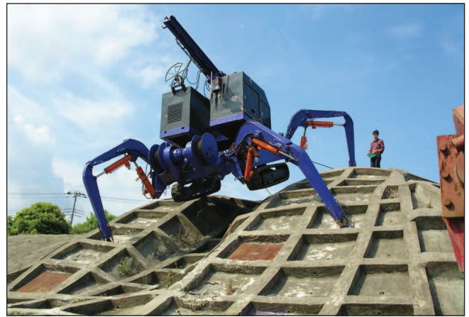
Figure 20. TITAN XI climbing up a test slope.
