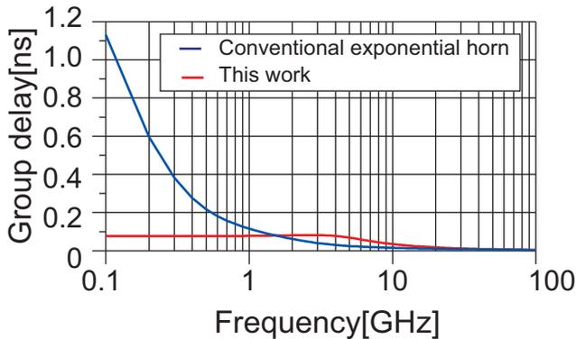
Fig. 11.  $S_{21}$  group delay characteristics. The proposed buffer shows a wide distortion-free region.
