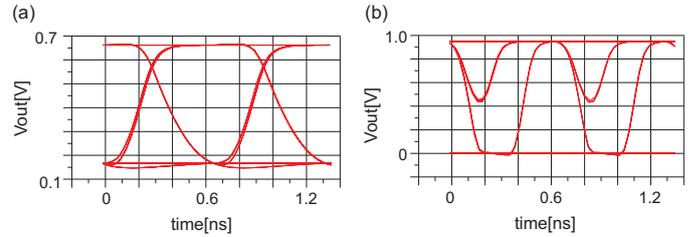
Fig. 13. Eye diagrams at 1.5 Gb/s when  $W_n = 1 \mu\text{m}$  and  $V_{\text{dd}} = 1.2 \text{ V}$ . (a) Proposed buffer. (b) Conventional buffer.
