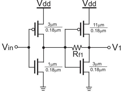
Fig. 7. Schematic of the first CMOS Cherry-Hooper stage.
