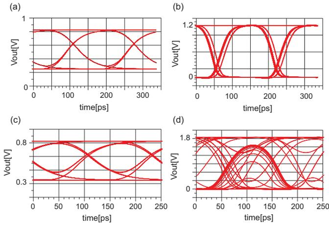
Fig. 9. Eye diagrams at 7 Gb/s [(a) and (b)] and 8 Gb/s [(c) and (d)].  $W_n = 1 \mu\text{m}$  and  $V_{\text{dd}} = 1.8 \text{ V}$ . (a) and (c) are results from the proposed buffer. (b) and (d) are results from the conventional buffer.
