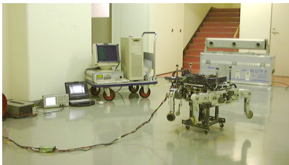
Fig.6.20 Experimental setup to measure the steering motion
