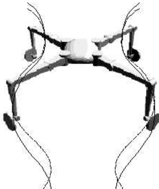
Fig.5.9 Roller skating locomotion
