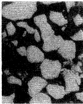
Photo. 8-3 Sectional view of magnetite particles within the partially reduced powder bed (z = 35 mm)
