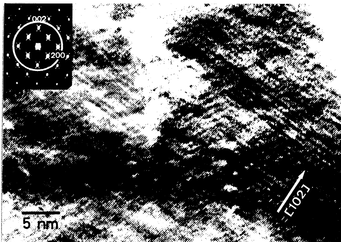
Fig. 4-2. [010]_{\alpha} , high resolution electron micrograph of a thicker part of specimen. White bands due to modulated structure are observed in two directions. Objective aperture size is indicated in the attached diffraction pattern.
