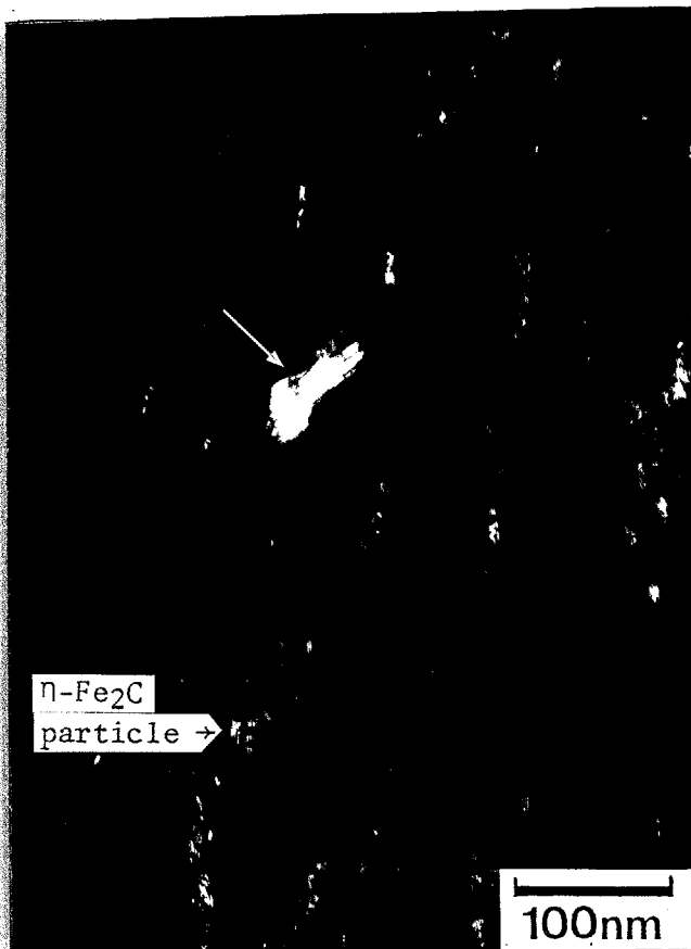
Fig. 5-2. Dark field image of \eta -Fe 2 C using 10\bar{1}_\eta reflection at the transitional stage from the first stage of tempering. Specimen : 1.5 mass%C tempered at 470 K for 50 hr. The particle marked by arrow is a \theta' -particle.
