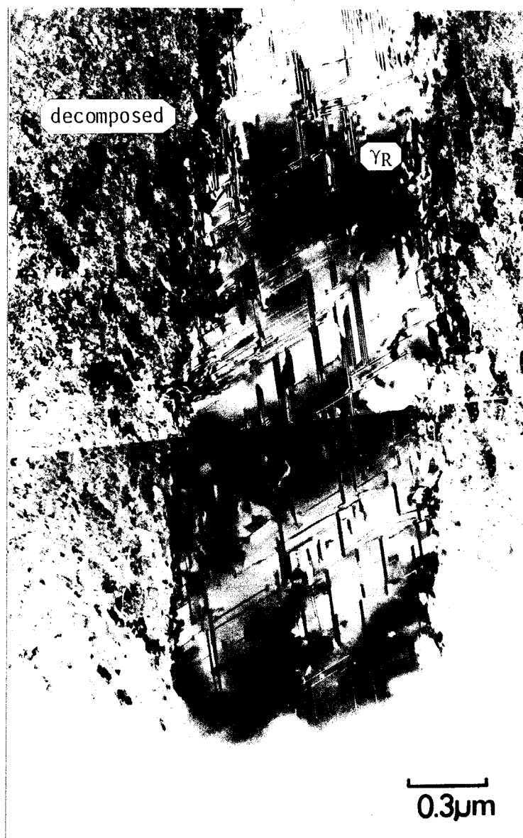
Fig. 6-8. Electron micrograph showing formation of stacking faults in retained austenite aged at 450 K for 10 days.
