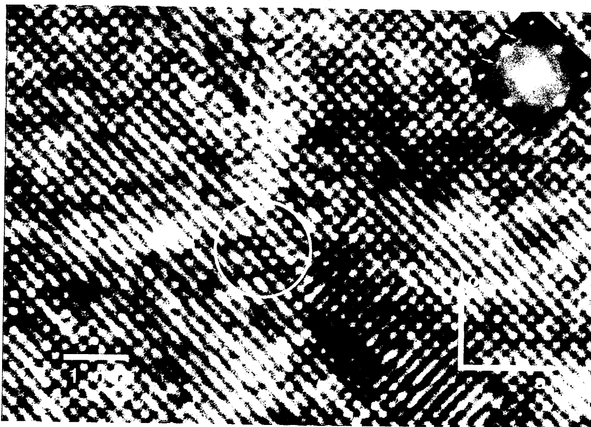
Fig. 4-18 High resolution electron micrograph showing the transitional state from the preliminary to the first stage of tempering. Specimen 1.6mass%C tempered at 340K for 30 min.
