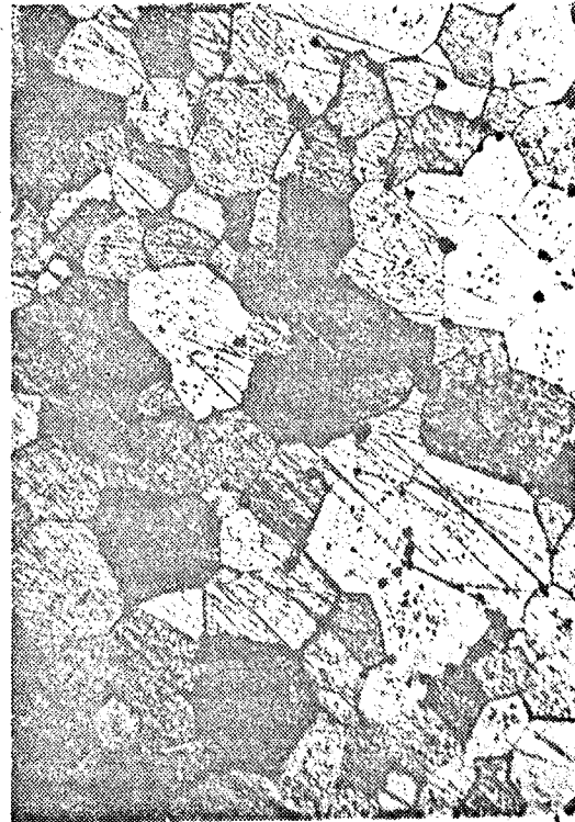
Photo 2-3 Grain Growth at 1620°C (0.2% Li 2 O)
