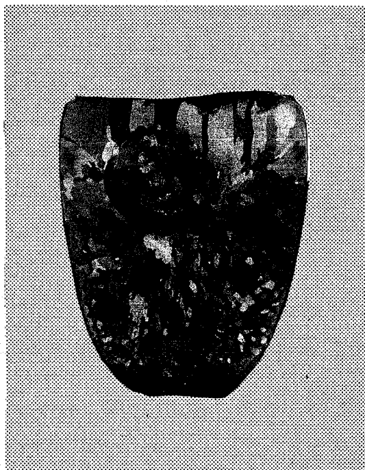
Fig. 7.1 Macro- and microstructure showing gravity segregation in Al-10 mass%Pb alloys solidified non-directionally.
