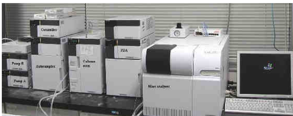
Figure 2.2 Photography of LC/MS system
