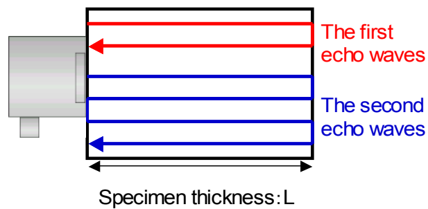
Fig.1.14 Schematic diagram of the two kinds of echo waves
