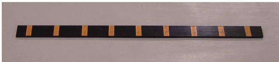
(b) Cross-ply laminate with nine electrodes
