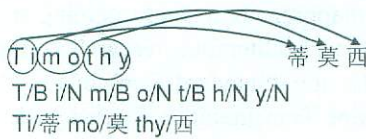
Figure 2: An pictorial description of a CRF segmenter and a CRF converter
