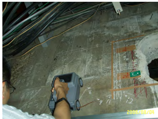
Fig. 5.4: Appearance of microwave radar survey
