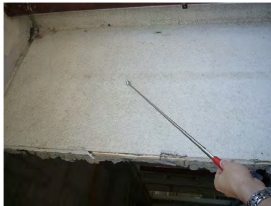
Fig. 5.2: Appearance of hammering test for debonding concrete wall
