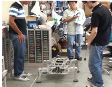
Fig.3 Walking experiment using TITAN-VIII
