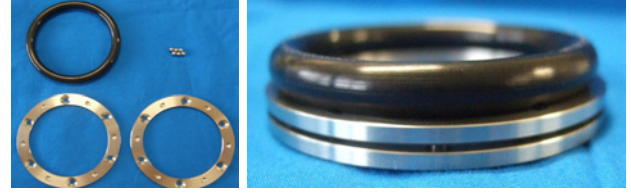
Fig.6 A prototype of proposed torque sensor
