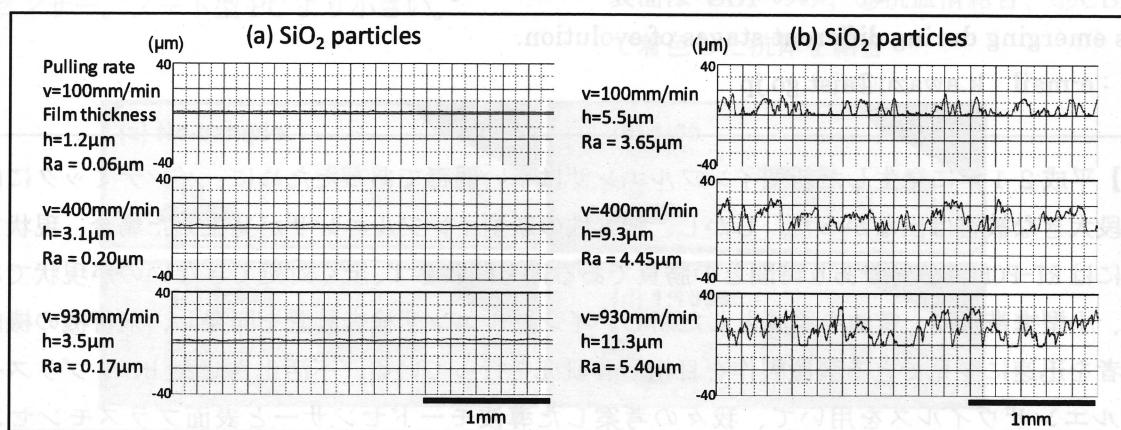
Fig. 2 Surface profiles of silica particle added films.
