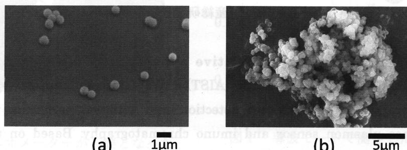
Fig. 1 SEM images of  $\text{SiO}_2$  particles.
