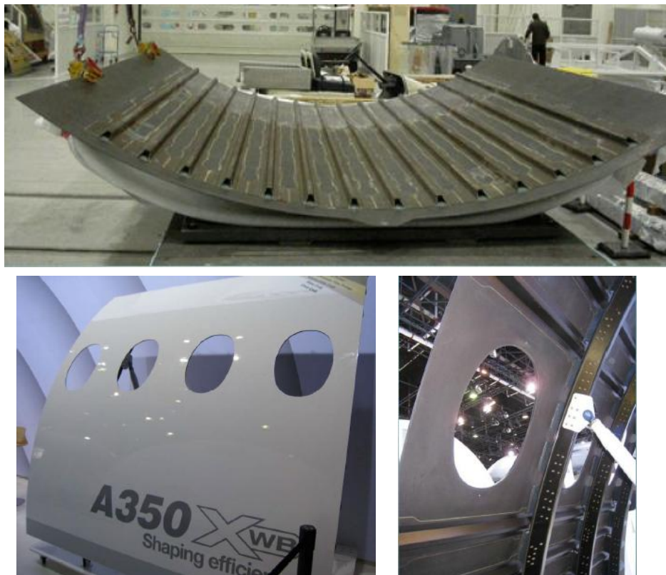
Fig. 2.12 Full composite fuselage of the Airbus A350 XWB (upper), demo parts of side panels (2,14) .
