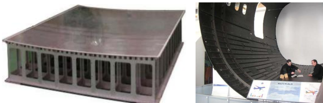
Fig. 2.11 Center main wing of the Boeing 787 (thickness: 6–20mm, mold dimension: 6m×6m×1.2m) (left), fuselage (right) (2,14) .
