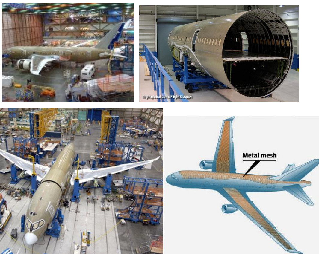
Fig. D.1 Lightning protection shield for Boeing 787 structures by acting as electrical paths for lightning strikes.
