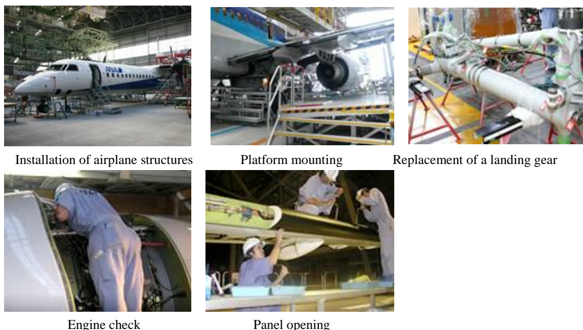
Fig. 1.11 Dock check for commercial aircraft structures (1.14) .
