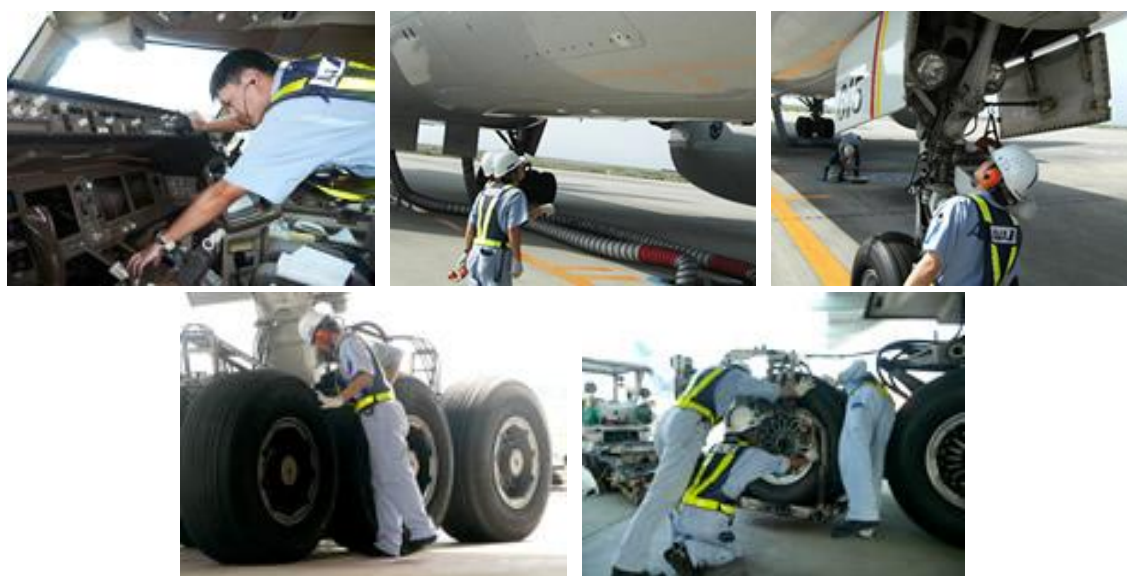
Fig. 1.10 Through flight check for commercial aircraft structures (1.14) .
