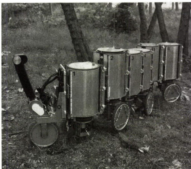
Fig. 7 KR-II moving over an uneven terrain
