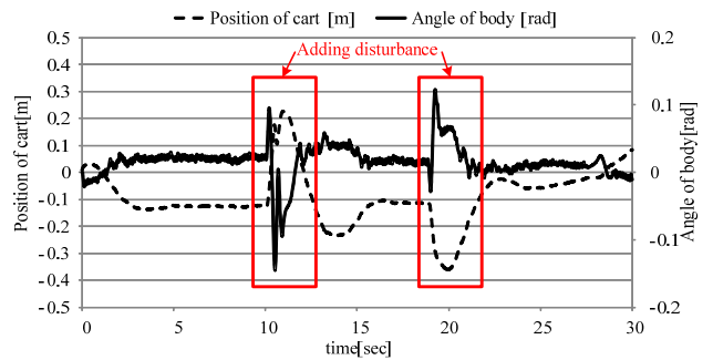
Fig.11 Experimental result of the attitude and position control
