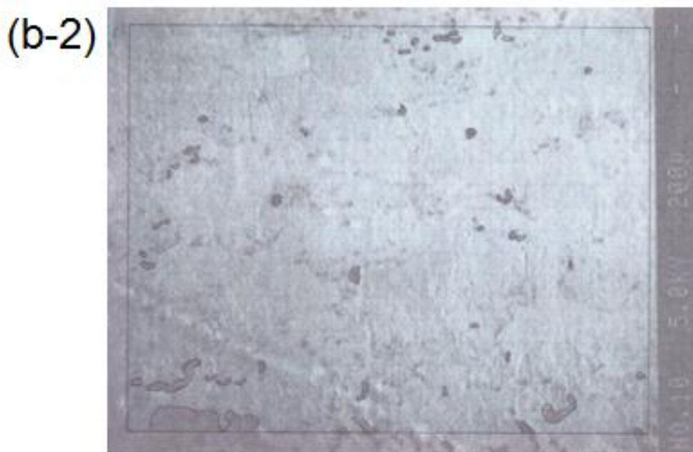
Fig. 3.28 Images of surface of reduced FeO for 960 s in Ar-5% \text{H}_2 -0.6% \text{H}_2\text{O} gas mixtures. (a) BE images (b) for measurement of coverage of reduced Fe.
