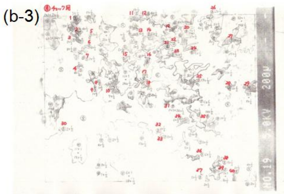
Fig. 3.30 Images of surface of the reduced FeO for 960 s in Ar-20% H_2 -0.6% H_2O gas mixtures. (a) BE images (b) for measurement of coverage of reduced Fe.
