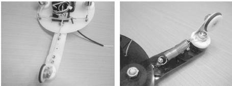
Fig. 10 Modification of the elastic elements
