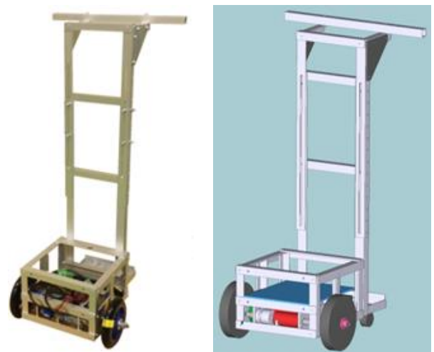
Fig. 7 Developed prototype mobile robot and its design
