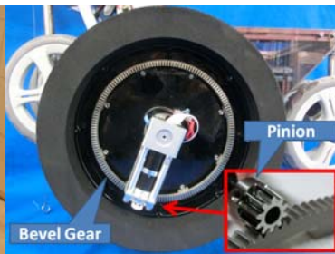
Fig. 4 Improvement of drive system
