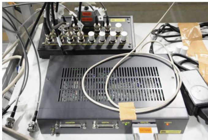
図 3-2-6 Digital Signal Processor (DSP) (mtt 社製・s-BOX)
