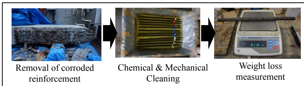
Fig. 2-4 Overview of corrosion weight loss measurement
