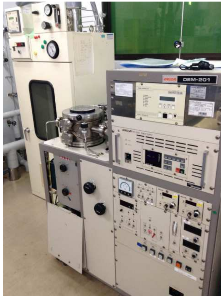
Fig. 3.6: Image of RIE system with \text{SF}_6 gas
