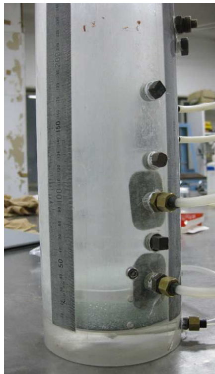
Figure 3.2 Photography of seepage test cell
