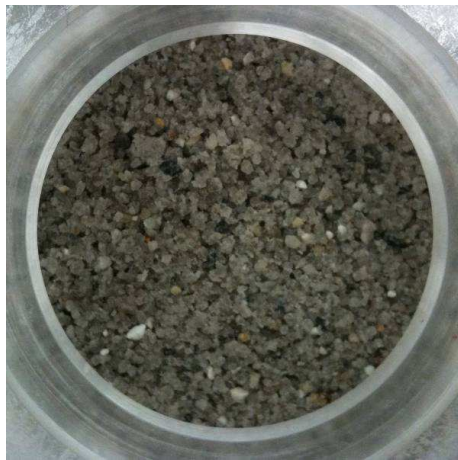
(a) Before internal erosion
