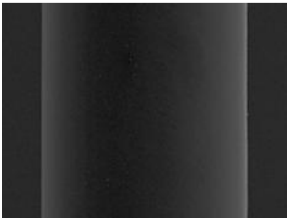
Figure 1-3. SEM photograph of smooth surface synthetic fiber produced by melt spinning.
