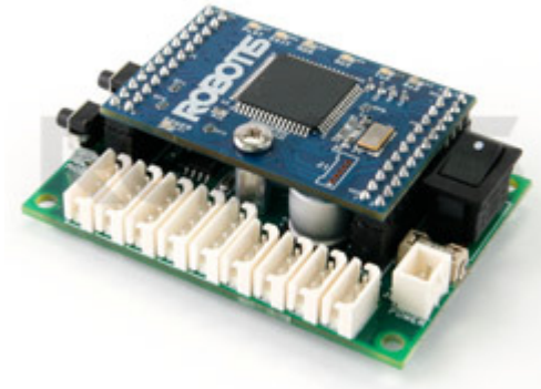
Figure 2.13 Main controller of the robot 'CM-700' [83]
