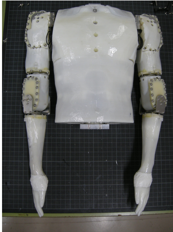
Figure 5.10 Remodeled upper body for free swimming
