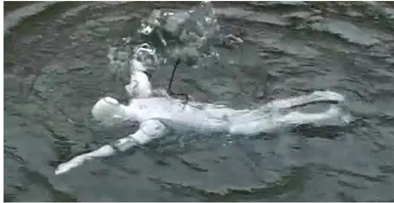
Figure 5.20 Abnormal recovery stroke during the experiment
