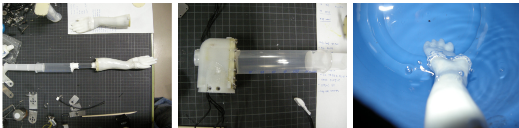
Figure 5.5 Waterproofing test by air injection
