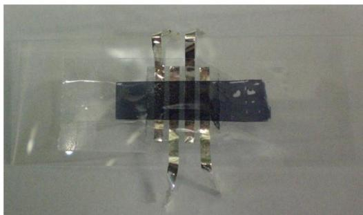
Fig. 3-10 Photograph of sample for four-probe method.
