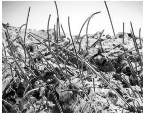
Figure 2.2 Fracture surface of FRC (ACI 544.1R-96, 2002)
