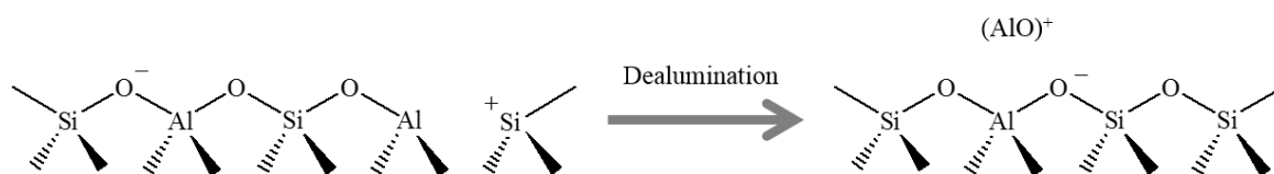
Scheme I-3. Framework dealumination of proton-form following Scheme I-2.
