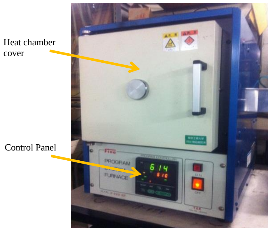
Figure 3. 3 Electric furnace used for annealing process
