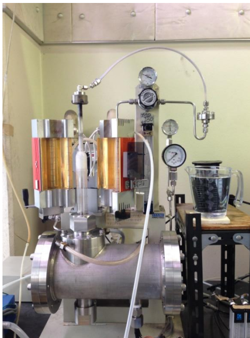
Figure 2.3 Photograph of the thermobalance with infrared gold image furnace.
