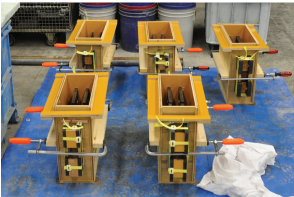
(a) Formwork for UFC segments
