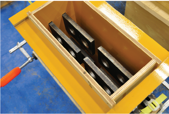
(b) Close-up of formwork for UFC segment
