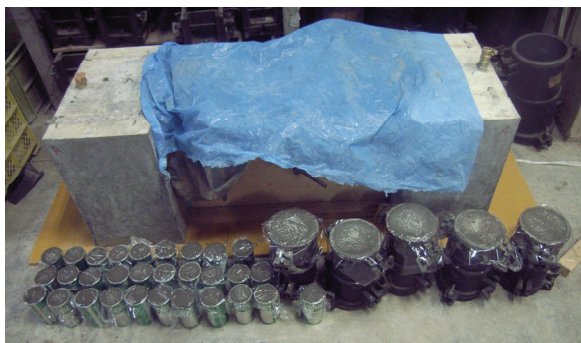
(f) Curing of specimen
